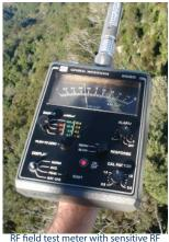
field test meter with sensitive RF cone attachment
