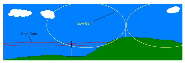
The above diagram demonstrates the effect of using a hi-gain antenna in a valley, **NOTE:** the beam with is narrow, and unable to reach the hilltop above.
