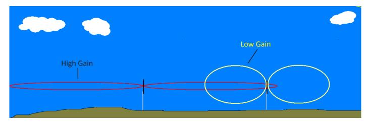
This diagram visualises the use of a Low-gain antenna, note that the beam width is significantly shorter and unable to reach the RF destination in addition RF energy is being waisted radiating into a wide beamwidth.
