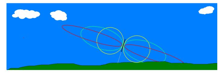
This diagram visualises the effect of an antenna that is not mounted in a vertical position. **NOTE:** that the RF transmission is radiated toward the Earth and Sky
